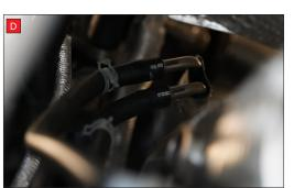
B) Feed Lambda cable down the right hand side (as you look at the engine). Ensure Lambda cable misses the gear cables, pass to the right hand side (as you look at engine). Take Lambda cable under the engine. Fit probe into Sensor boss on the downpipe and tighten.
