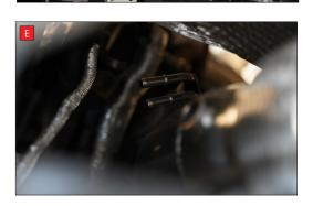
C/D/E) Locate the 2 GPF pressure sensor lines (Image C shows them with the downpipe removed for better view). Remove the clamps and pull the rubber hoses from the metal hard lines. Place the 2 vacuum blanking caps over the open ends of the hard lines to seal them.
