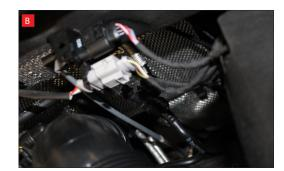
A) Remove Lambda Probe from OE catalyst, then remove cable from clips indicated. (x4)
